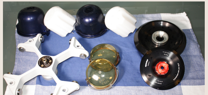
Figure 4: Clean rotor and rotor bores with plastic scrub pad and/or stiff test-tube brush in case of stubborn stain. Then rinse with water and dry.
