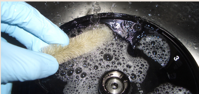
Figure 4: Clean rotor and rotor bores with plastic scrub pad and/or stiff test-tube brush in case of stubborn stain. Then rinse with water and dry.
