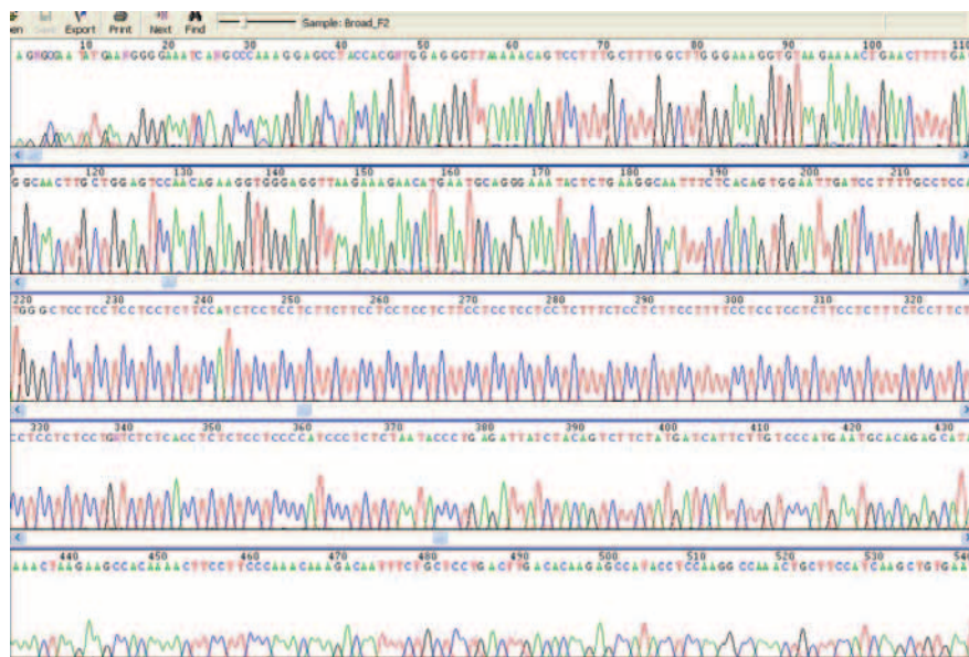
Fig 5. Electropherogram of a TC-rich region of a fosmid template after amplification with the illustra TempliPhi Sequence Resolver Kit shows that there is no need to use additives to successfully resolve such a difficult region.
