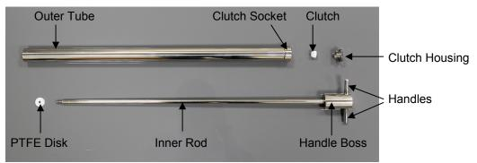
Materials of Construction: Inner Rod: 316 stainless steel
