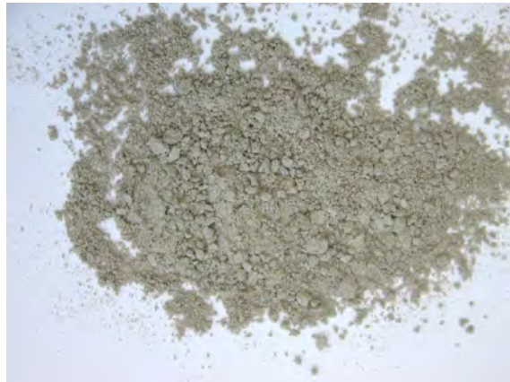
Fig. 2: after grinding in MM 200
