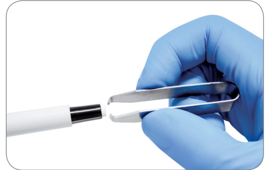
Removing the Safe-Cone Filter
