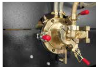
Equipment flanges can be furnished with fast clamping seals.
