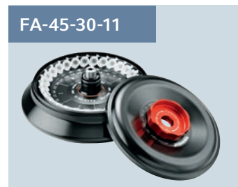
FA-45-30-11 30 x 1.5/2 mL micro tube rotor with aerosol-tight lid for safe centrifugation of hazardous samples. Max. speed 20,800 x g (14,000 rpm).
