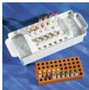
The larger rack has a tray that can be used as an ice bath.
