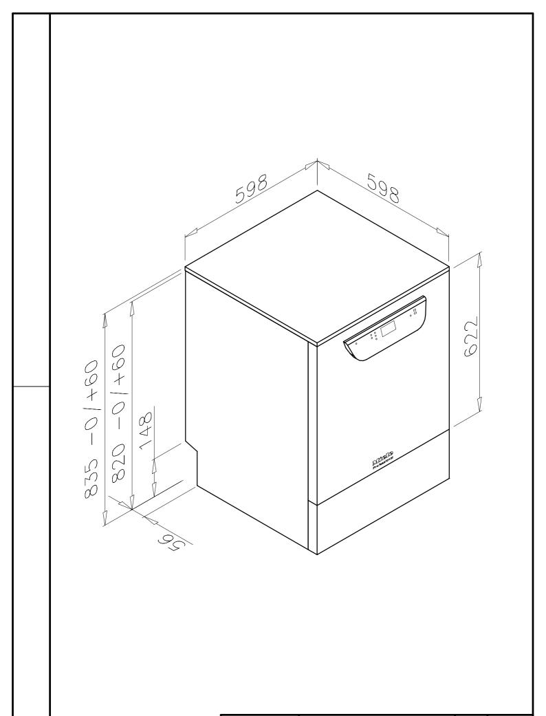
Míele PROFESSIONAL Installationsplan/Installation plan Thermo—Desinfektor PG 8582 — PG 8583
