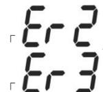
'Er2' is displayed when the thermometer is exposed to rapid changes in the ambient temperature. 'Er3' is displayed when the ambient temperature exceeds 0°C(32°F) or +50°C (122°F). The thermometer should be allowed plenty of time (minimum 30 minutes) to stabilize to the working/room temperature.
