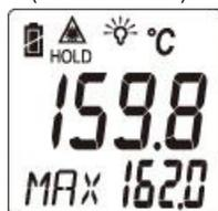
1. Simply aim the thermometer at the measure target with Lens (④) and press Meas. key (⑥) to display the surface temperature.
