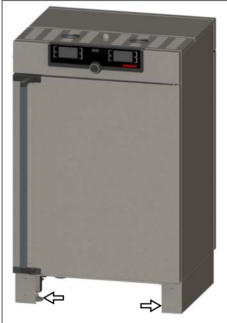
Fig. 10 Screw the appliance to the housing base by the adjustable feet
