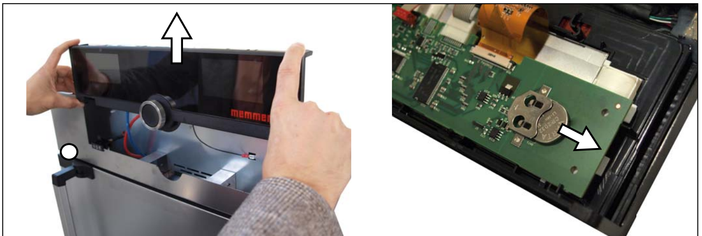
Fig. 23 Removing the lithium battery
