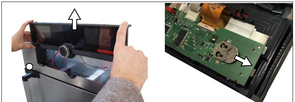
Fig. 26 Removing the lithium battery
