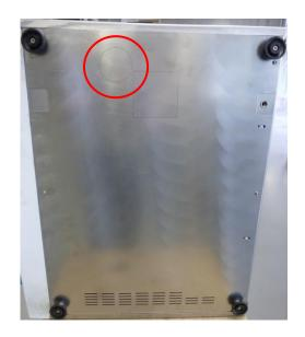
Remove the round pre-cut part from the bottom plate.
