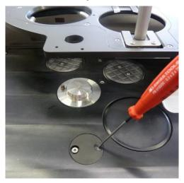
Remove the two plastic screw caps and remove the dummy cover on the rotor slide plate.
