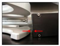
Mount the rotor to the MEDIAJET and check whether the clearance between the rotor and the printhead is between 1.5 to 3.5 mm.
