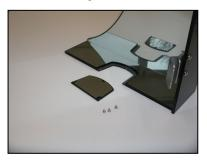
Remove the slot cover on the back side of the MEDIAJET Plexiglas safety cover.
