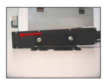
Place the printhead on a flat surface and adjust the adapter plate so that the head points slightly downward. Completely tighten the two Allen screws.
