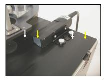
Fix the printhead onto the MEDIAJET with the two knurled head screws.
