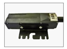
Fix the printhead adapter to the MI inkjet printhead using the two M6x10 Allen screws.
