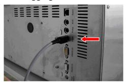
Insert the Mini-DIN 8 poles plug of the Interface cable (103081) into the socket labeled with INKJET on the rear panel of the MEDIAJET.
