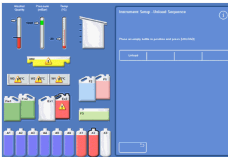
Unloading clearants – Ex2 full and X2 outlined
