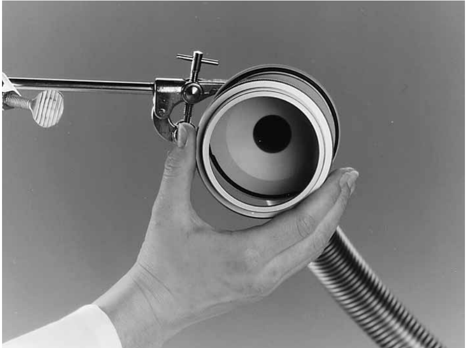
Fig. 7 Use the clamp 17037 and clamp holder 16976 to fix the connector on the stand 16970.
