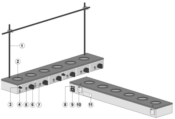
**7.2.2.** Switch on the mains electrical supply. Adjust the controller regulator knob in each position to the required setting.
