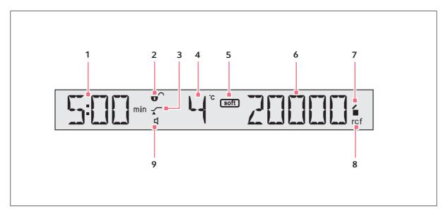
Fig. 5-2: Display of the Centrifuge 5424 R, similar to the display of the Centrifuge 5424.
