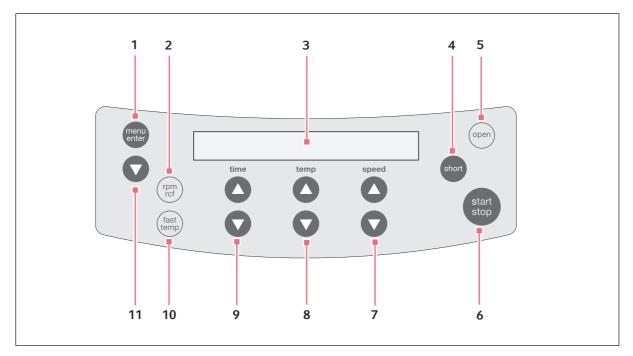
Fig. 5-1: Control panel of the Centrifuge 5424 / 5424 R
