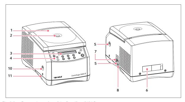
Fig. 2-2: Front and rear view of the Centrifuge 5424 R
