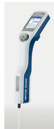
Figure 3: A digital hydro-meter. In this case, the METTLER TOLEDO Density2Go instrument.
