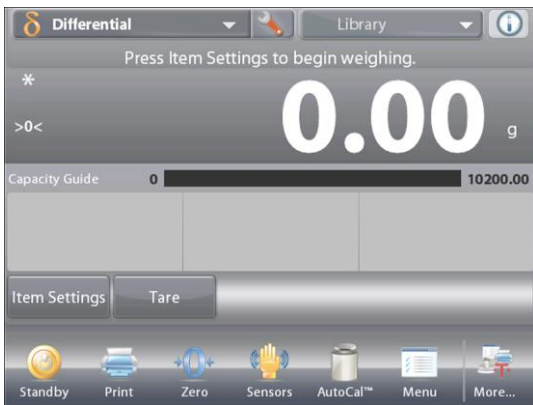
The DIFFERENTIAL WEIGHING – Auto Home screen
