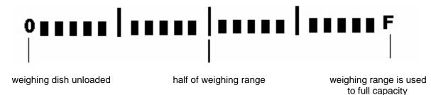
The weighing range of the balance is divided into 20 graphic cuboids. Zero (0) will appear on the graphic display if there is no weighing value on the balance. 10 graphic cuboids are displayed if the balance is loaded up to one half of its weighing range.
