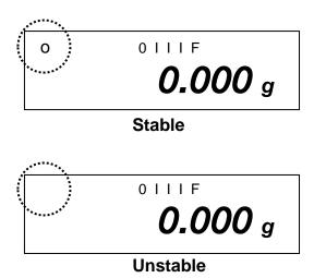
The balance is in a stable condition if the [o] stability indication appears on the display. The [o] indication disappears if the condition is unstable. Stable ambient conditions can be achieved by using the draft shield (See chap. 5.2.4 for installation)
