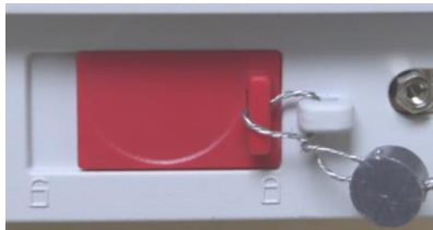
Locked with Wire Seal
