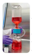
Stericup® E and Steritop® E filters thread directly onto any commercial media bottle or glass bottle:
